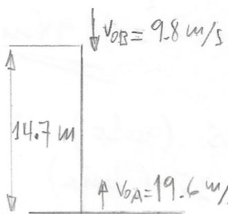
$$\left. \begin{aligned} e_A &= V_{0A} t - \frac{1}{2} g t^2 = 19.6t - 4.9t^2 \\ e_B &= V_{0B}(t - R) + \frac{1}{2} g (t - R)^2 = \\ &= 9.8(t - R) + 4.9(t - R)^2 \\ e_A + e_B &= 14.7 \end{aligned} \right\}$$
